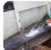
Liquid penetrant testing
