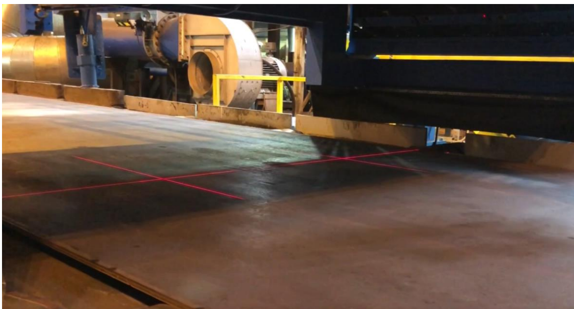
Fig. 2 – GEOMETRIX-PL. Laser projection lines seen on material in-line
